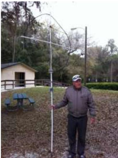
**Art WB4MNK #5274** used his Elecraft KX1 running 3W, used a Dirt Cheap paddle, and brought out his new toy, a homebrewed magnetic loop antenna (that was matched with a 1.2:1 SWR).
